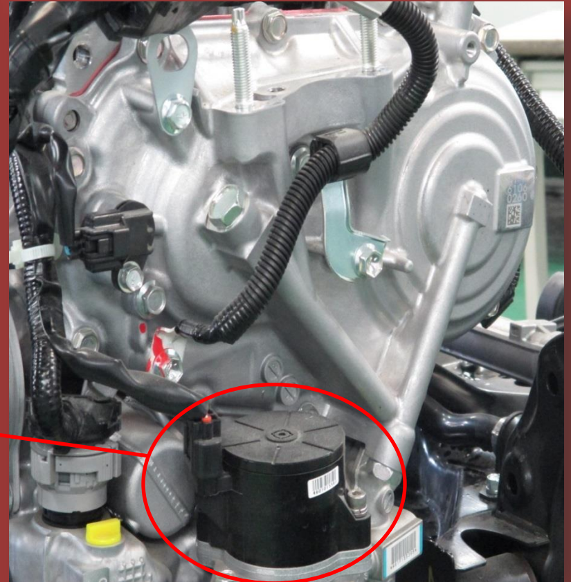
Electric pump for Idling Stop
